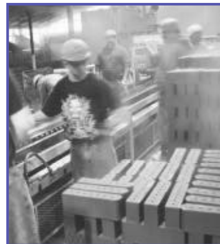
Bricks are cut by machine and stacked by hand, ready to go to the kiln
